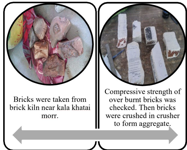
Fig. 1. Preparation of over burnt brick ballast from over burnt bricks
