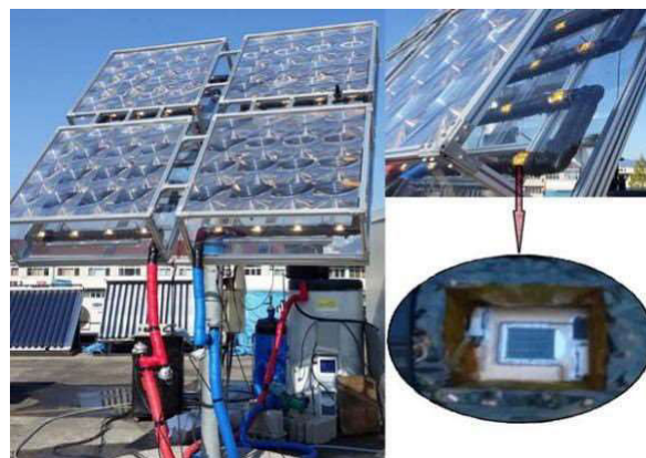
Fig.11. Concentrated Photovoltaic Cogeneration system [29]
